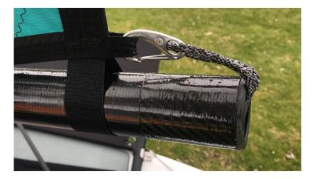
2. On the topside of the boom there is a clam cleat, the rope passes through this and can be adjusted as necessary.
