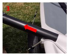
The wing covers are supplied fully assembled, laced together with cable ties. Should the covers need replacing, these ties are easy to cut off and replaced. Only use UV stable Nylon with at least 50Kg breaking load.
