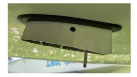
2. Attach the horizontal main foil under the boat whilst on the trolley by aligning the pins, press the push button in and slide the foil it up into place.
