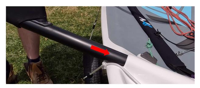
2. Lower the rear bar into position and push the bar over the inner pin.
