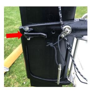
2. Attach the horizontal foil by aligning the pins, press the push button in and pushing it up into place. Make sure the push button is fully engaged before going sailing. The button will sit flush on the outside surface of the rudder.
