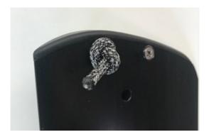
4. The excess rope can be hooked over the knob at the end of the tiller.
