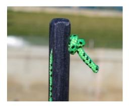
The wand is now ready for use, pull the cord to raise or lower the wand. This changes the ride height whilst sailing.
