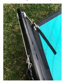
3. Run the excess rope through the halyard keepers on the front of the mast.
