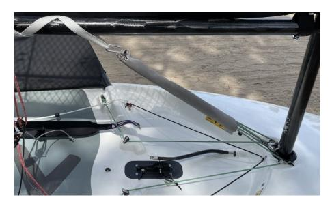
1. Attach the snap shackle to the mast saddle. Be sure to not twist or tangle the ropes.
