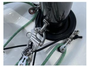
2. Attach the hook onto the boom vang loop.
