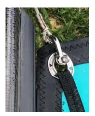
2. When the sail is fully raised, insert the swage into the halyard lock on the front side of the mast.
