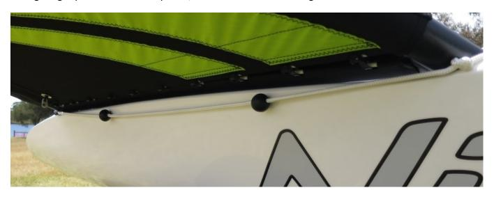
To remove wings: Undo the retaining fast pin (1), lift the rear wing bar up and pull it away from the hull to clear of the 2 attachment pins (2). Then slide the front wing bar outwards and away from the hull (3).
