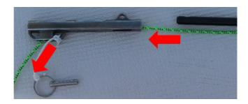
2. Insert the wand inside the wand tube assembly, ensuring the rope is sitting in the groove at the back of the wand.
