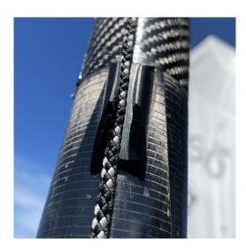
4. Cleat the rope onto the horn cleat near the base of the sail track. The remaining halyard rope can be stored in the sail pocket.
