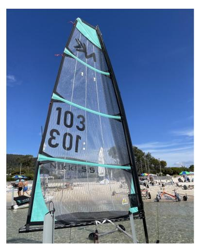
1. Insert the head of the sail into the sail-feeder and feed the luff up the sail track on the back of the mast and attach the Halyard shackle to the eye at the head of the sail.
