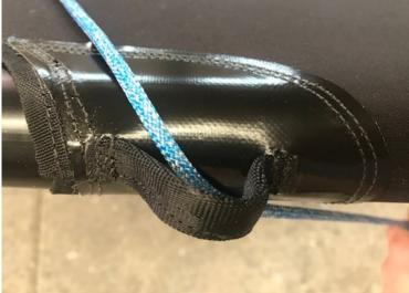
2. On the underneath side of the wing (where the yellow stripes are) near the aft and inner wing bar, there is a sister clip. Pull both sister clips together and connect them.
