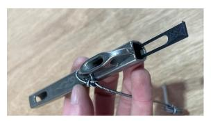
2. Position in place and insert the wand to hold the spacer in place as the glue dries. Make sure the cutout lines up with the rope feeder.
