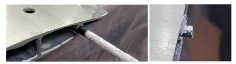
10. To put in all the plugs, squirt some more Sikaflex into the cavities. It can help if you can extend the nozzle to be able to get the Sikaflex up further. We use a plastic tube and tape it onto the nozzle.
