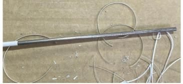
5. Test fit the 100mm piece of tube to make sure it slides nicely on the pushrod.
