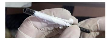
9. Insert the fiberglass tube put in until about 5mm from the end of the daggerboard.
