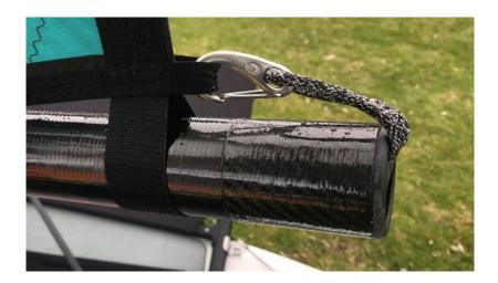
2. Insert the yoke end into the webbing loop on the tack of the sail and clip the yoke onto the mast. Ensure the webbing is positioned in front of the boom hook.
