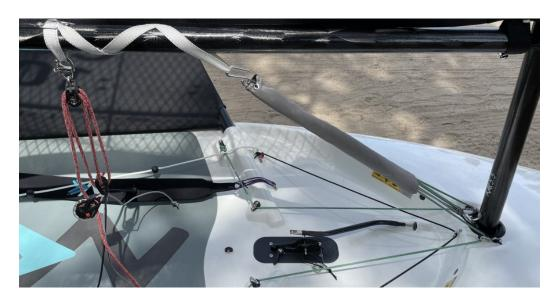
1. Attach the snap shackle to the mast saddle. Be sure to not twist or tangle the ropes.
