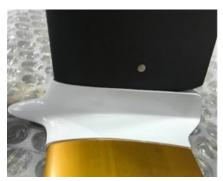
Make sure the push button is fully engaged before going sailing. The button will sit flush on the outside surface of the rudder.
