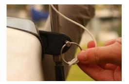
4. Run the wand rope around the boat, threading the wand cord through the fairleads and pulleys as shown below.
