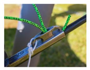
6. Insert the tail of the wand rope in the top wand hole and tie a knot to the correct tension.
