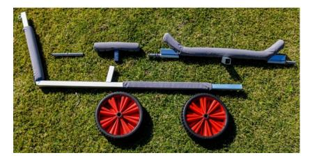
1. To join the trolley centre bar and the trolley rear bar together, push the spring clip in and insert the centre bar into the square tube on the trolley rear bar. The spring clip will click into the hole.
