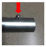
3. To attach the wheels, place the wheels onto the axle, then place the washer over the axle. Insert the linch pin into the hole on the outside of the axle.
