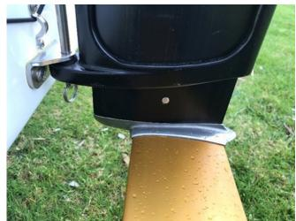
3. Insert the pull-down rope into the hole on the top of the rudder and tie a knot. The rudder is pulled down into place using this rope after leaving the shore.
