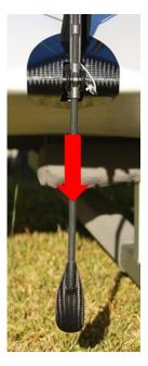
1. Thread the rope through the wand tube and out the slot in the back of the wand tube.
