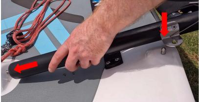
3. The outer pin will sit inside the hole on the bracket attached to the rear bar. Push the retaining pin in place.
