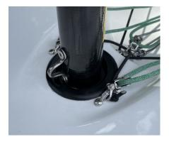
Once fully down, rotate the mast 180degrees to its sailing position with the sail track towards the stern.
