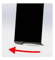
Rotate the knob anti-clockwise to reduce angle of attack on the rudder lifting foil, to sink the stern of the boat during foiling. The Rudder Pin will move towards the back of the slot.
