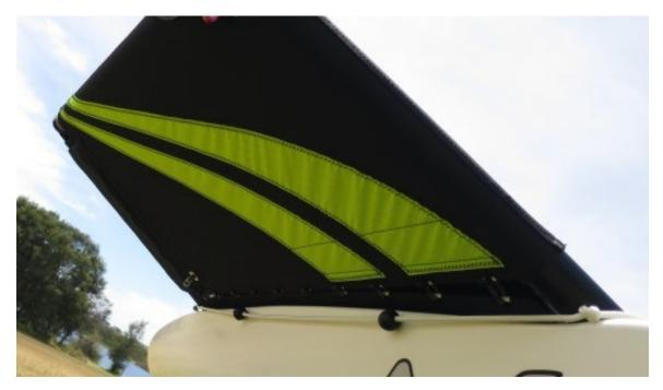
The underside of the wing covers have yellow stripes to help make the boat more easily visible when capsized.
