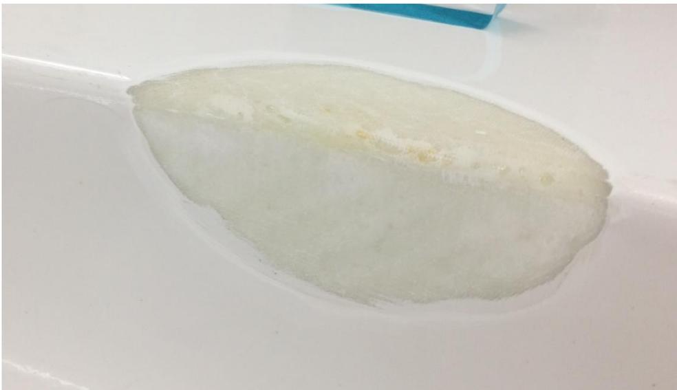
4. If there is a big puncture hole you will have to glue a piece of EPS foam in with epoxy, wait for it to cure and then smooth off to the correct shape.
