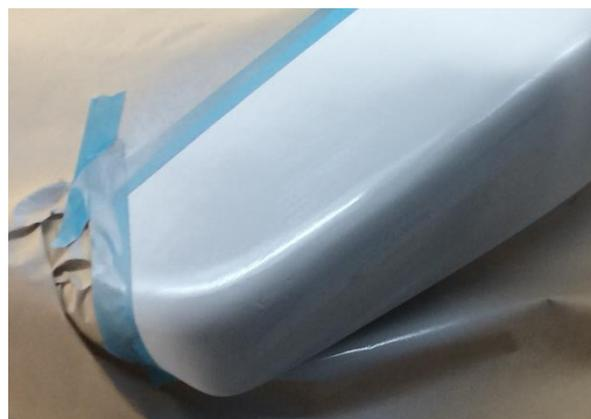
5. When dry, sand again with sanding block using 240 grit sandpaper, this time sanding even wider area again.
