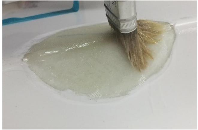
8. Add Peel ply on top of the layers, wet it out a little bit and use your putty card to squeeze excess resin out (you can skip this step if you don't have peel ply)
