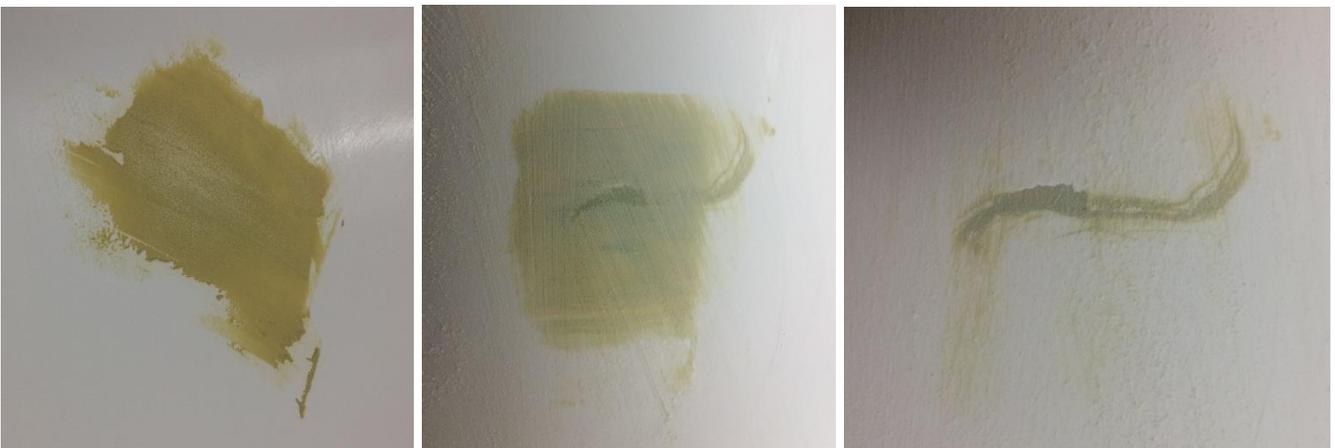
3. Do not overfill the area, it is much better to fill several times and sand with 100 grit and sanding block lightly between fills than to try and over fill the area and then sand it to the right shape. Otherwise, you may end up sanding a lot bigger area and take longer to get the correct fairness and smoothness.
