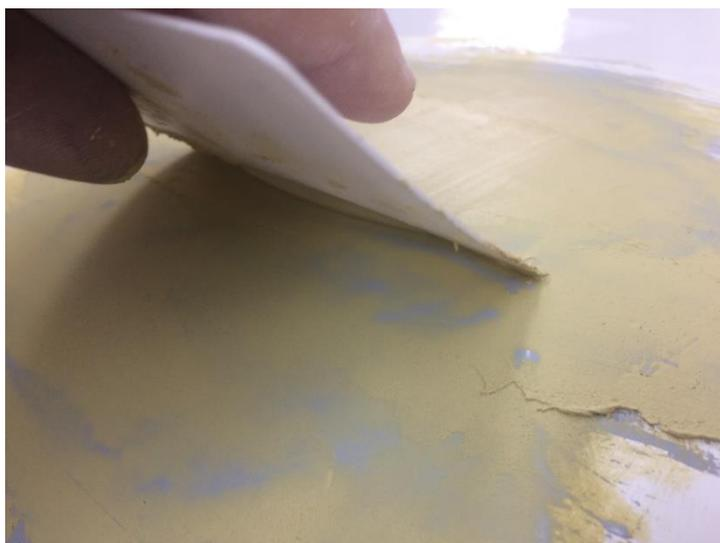
4. When the filler is dry sand with 180 grit sandpaper a little wider than before and apply another coat of high build surfacing primer, again making sure that all the sanding scratches are covered.
