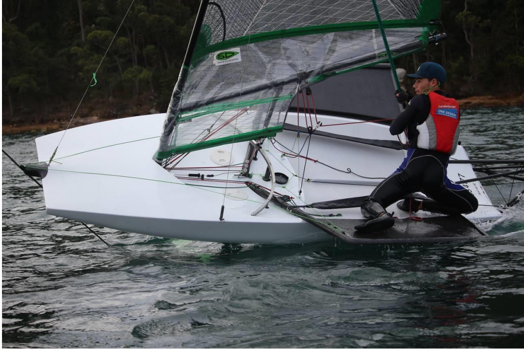
The Skeeta hull is wide and stable, making capsizes less likely and the boat inherently safer.
