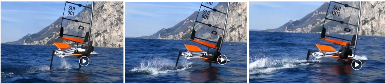
Riding too high, the main foil ventilates and begins to dive
